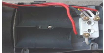
Step 3: After remove end cover, find the terminal connected to the capacitor lead, loosen the fastening nut and remove the original wire of capacitor and motor.
